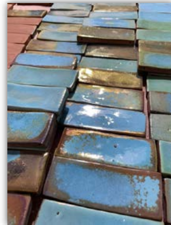
Figure 10: the units the second firing (glaze firing) at temperature 1050°C
